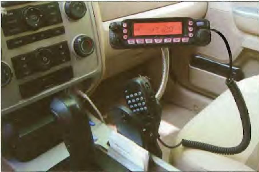
Figure 4 — A cheap solution to a no holes mount installation. Note how the unit is clamped to the center console and also the position of the microphone clip.
