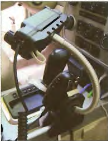
Figure 5 — A rear view of the no holes mount attached to the center console and showing the microphone clip installed on the lamp base.
