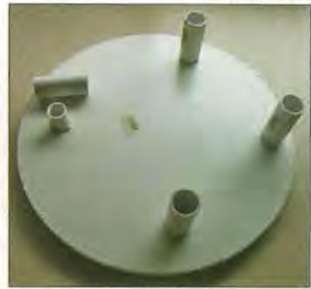
Figure 6 — The underside of the table showing the added PVC caps and tubing "legs."
